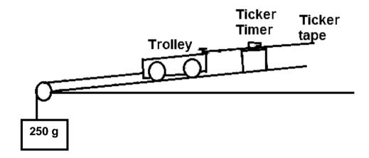
The runway was inclined to compensate for friction. The mass piece accelerated the trolley down the incline. The incline was kept constant for the duration of the experiment. The mass was increased by stacking the trolleys one on top of the other after each reading. After analysis of the four ticker tapes, the following results were recorded:
